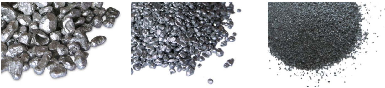
Fig. 2 Different grades of Aluminum (left to right: coarse [approx. 10 mm], medium [approx. 3 mm] fine [approx. 500 µm])
